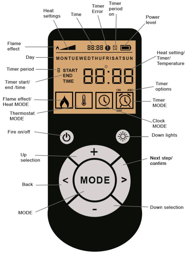
**!** **Timer Error** - Displays when the END time is set before start time. Also displays when 2 or more timer periods overlap.
